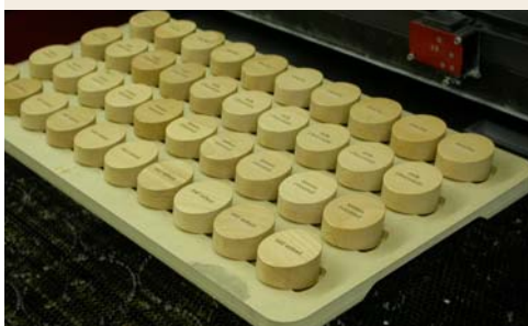
Hundreds of wood pucks lasered in a custom fixture.
